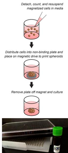
Top: Schematic of magnetic 3D bioprinting spheroids.<sup>2</sup> Bottom: 384-well Bioprinting Kit with NanoShuttle, spheroid drive, and non-binding microplates
